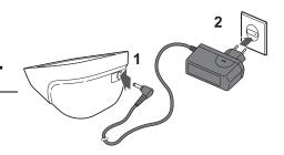
To disconnect the AC adapter, unplug the AC adapter from the electrical outlet first and then remove the AC adapter plug from the main unit.
