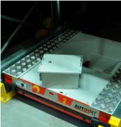
Longlife lithium battery removed for recharging
