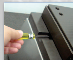
Setting Amplitude of Sample Sweep
