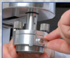
'Quick Release' Sample Interface
