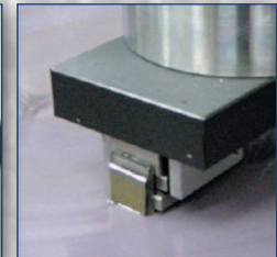
6145.1 Single Die Stub Cross-section holder
