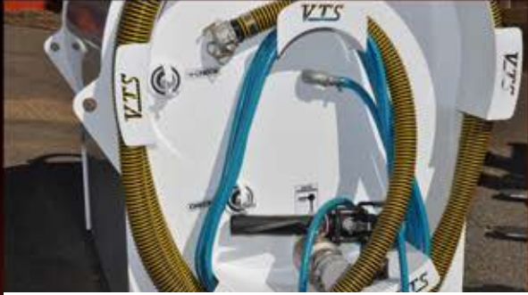
SUCTION AND WATER HOSES FITTED
