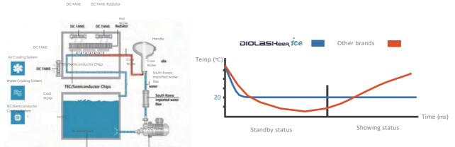
The instrument is internally loaded with a TEC refrigeration system and an intelligent temperature monitoring sensor to ensure that the operating temperature of the machine is constant at 20 degrees Celsius. Ensures that the water temperature remains the same for 24 hours of continuous operation.
