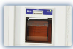
Recorder supports the print of 3-channel waveform at the same time. ( Optional )
