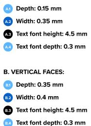
Embossed features are extruded from the surface of the model. Small embossed features may not be visible on the finished part. Use a bold font where possible for best results with embossed text.
