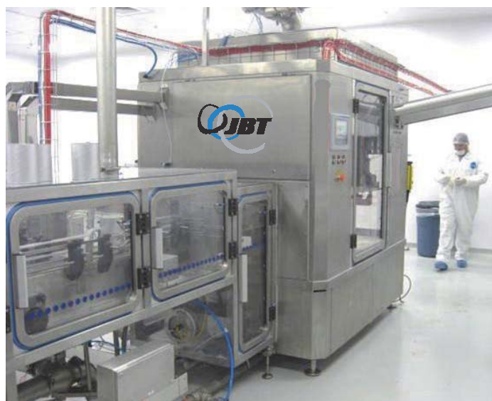
▲ JBT SeamTec™ Pre-gassing Closer with gas-tight guarding
