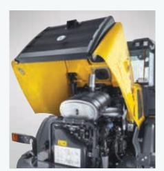
• One piece engine hood features electric opening on W130 D, W170 D and W190 D models
