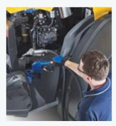
• For security, the fuel tank and AdBlue tank are accessed only by raising the engine hood
