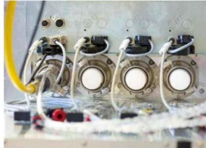
4-exit beam switch
