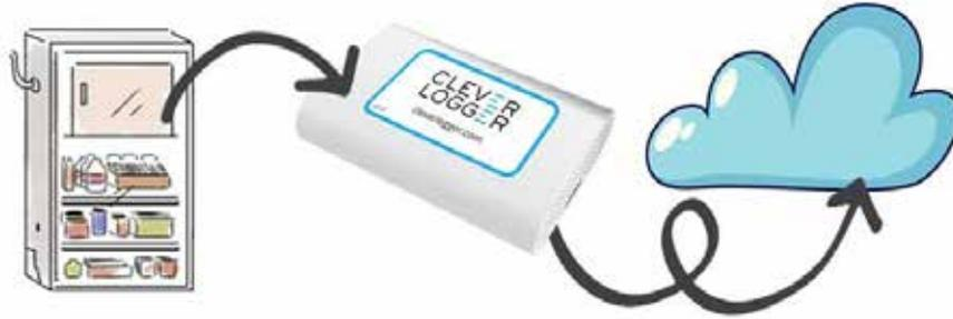
Clever Loggers are connected directly to the internet via a Gateway. The temperature in your fridge or freezer is recorded and saved to the internet every few minutes.
