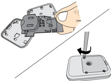
Return the circuit board to the logger, replace the cover and screw it down.
