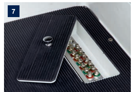
7 Accessible central lubrication at machine front
