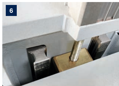
6 Linear guide for precise adjustment of the top spindles and optimal work piece quality
