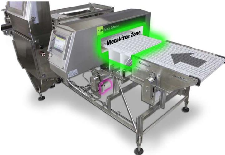
Conveyor motor (purple) is mounted away from the metal detector aperture ensuring EM fields do not interfere. A metal-free conveyor section (green) is needed to ensure metal is not near the aperture.
