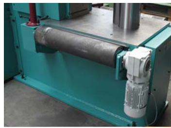
116 Driven roller directly at the machine
