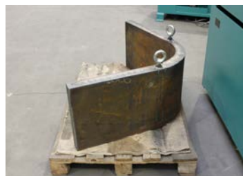
126 Heavy bending works e.q 400x60 mm
