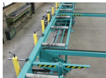
131 Laser measurement along the entire profile length, incl. creation of a report
