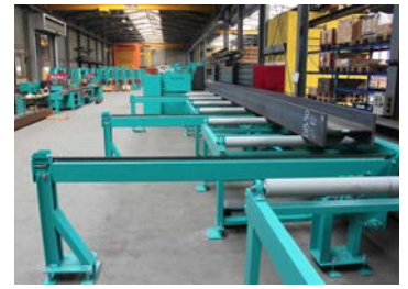
117 Cross conveyor system
