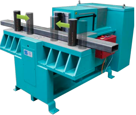
114 Straightening press with several straightening pins for bulky welded constructions
