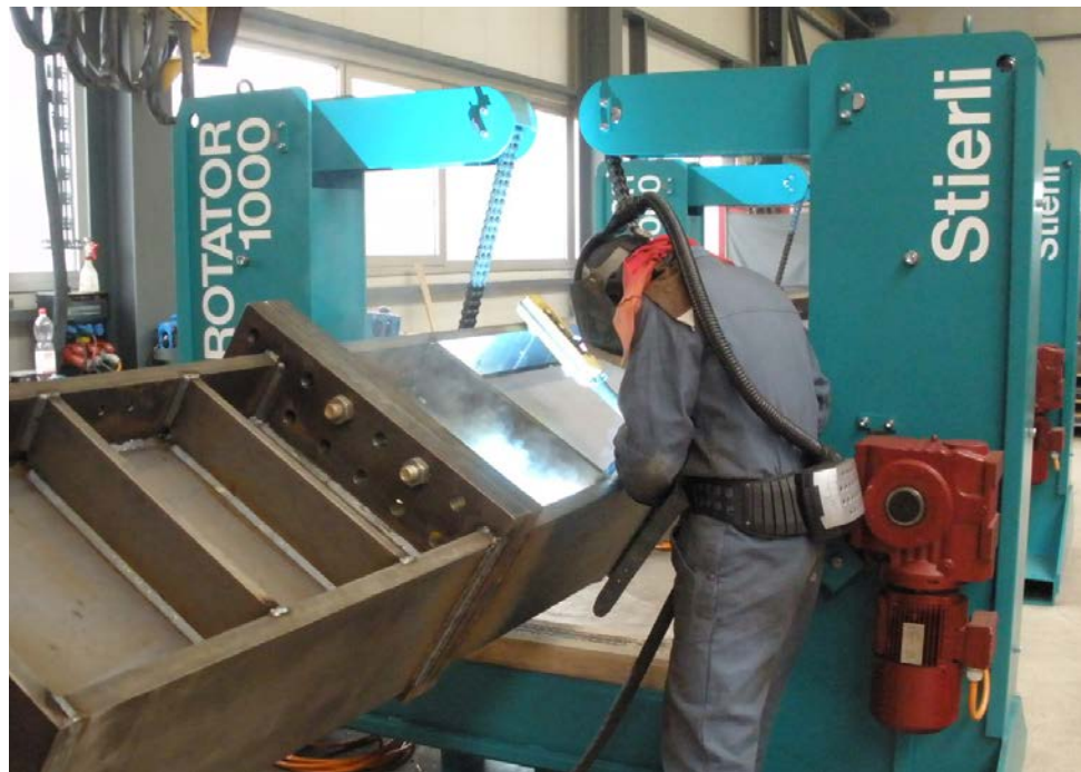
Welding in flat position increase the productivity
