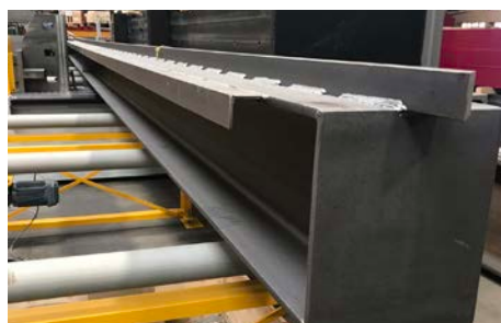
128 Crane beam straightening (instead of flame straightening)
