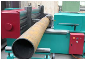
111 Pipe bending up to \varnothing 400\text{mm}
