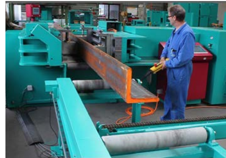
120 Straightening large L-profiles 300x300x30mm
