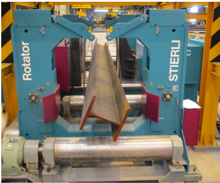
115 600 tons straightening press combined with ROTATOR for fast and safely turning of beams within the machine.
