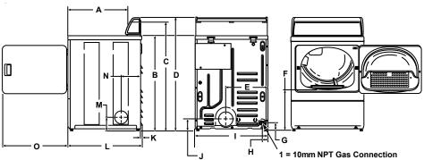
All measurements are in mm. \*With levelling legs turned into base.
