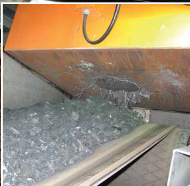
These images are two examples of manual-clean magnets pulling unwanted metals out of conveyed products.
