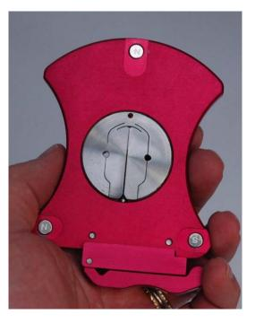
2.) While holding the polishing disk in place, secure the four mounting screws, but do not tighten, leaving the polishing disk free to rotate during the next step. Place two appropriately sized ferrules into the fixture to expand the flexure design.
