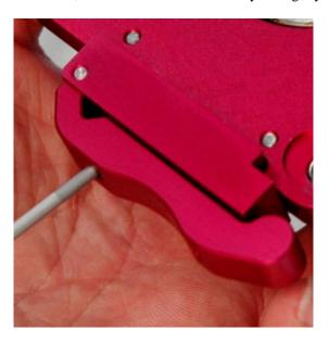
4.) Tighten the 4 screws to secure the polishing fixture in place, disengage the release handle, remove the inserted connectors, and now the fixture is ready to use.
