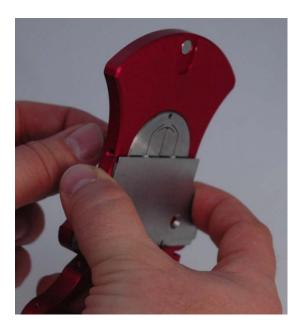
Note: If only polishing one connector, a dummy ferrule or connector must be used in the other hole. This dummy ferrule does not have to protrude through the bottom of the fixture; it is only needed to fill the space for the connector securing mechanism to function properly.
