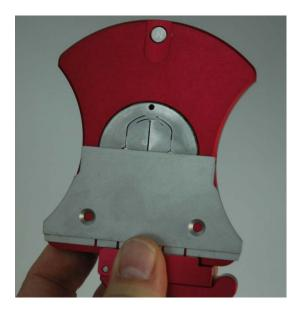
**6. Insert each connector** in the fixture until the ferrule end face contacts the reference plate (ferrule protrusion is ~1mm). For LC and SC connectors, do not use the reference plate at all and simply insert into fixture and lock. The ferrule does not protrude enough to contact the reference plate.
