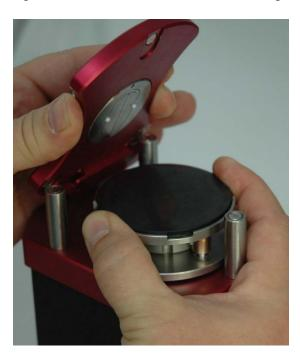
**13. Polish ferrules:** (See Section 10 for recommended polishing film schedule and polishing times for standard connectors.)
