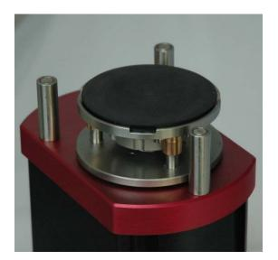
Note: Four pads are supplied so that each pad can be used for a different polishing film. To speed up your process times, place a different grit polishing film on each pad. This way when it is time to change the film for the next step, just place the pad with the appropriate film on the machine.
