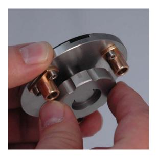
Note: There are two indicators on each knob. A full hash mark and a partial hash mark to indicate position when setting the spring force.
