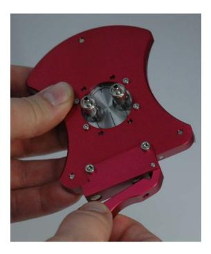
Note: The loaded PDH fixture can be placed on a flat surface without damaging the prepared ferrule end faces, since the release handle mechanism holds the ferrule tips off the table surface.
