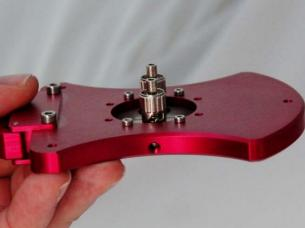
3.) Close the release handle. The release handle should not be touching main the PDH fixture, if it is then adjust the set screw to move the release handle slightly off the fixture. To achieve the strongest magnetic attraction, the release handle should only be slightly separated from the fixture.
