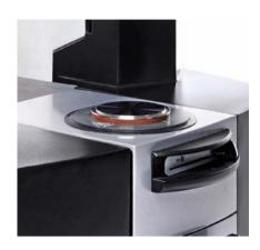
Environmental controller for cone-plate and plate-plate measuring systems
