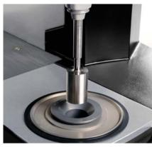
Environmental controller with concentric cylinder-type measuring systems
