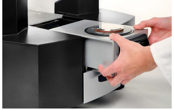
Environmental cartridges are easily interchangeable within seconds without the need to connect hoses or control cables
