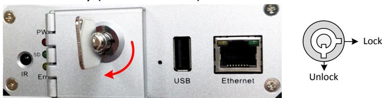
2. Lift up the card protection plate and insert a SD card into the SD Card slot (the lower one).
