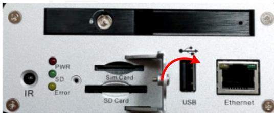
3. Restart the MDVR for detecting the SIM card.
