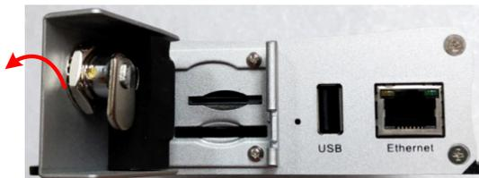
3. Restart the MDVR for detecting the SIM card.
