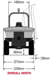
MAX SAFE CARRYING WEIGHT: 6000KG | LEVELLED CAPACITY: 2400L | HEAPED CAPACITY: 3200L
