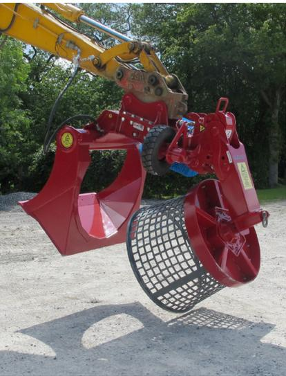
Interchangeable drums, from 10mm to 100mm, with cleaning brush fitted as standard.
