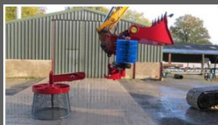
Unique drum change system on larger buckets offering users the ability to produce varying sized materials throughout the working day with ease
