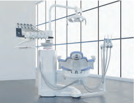
S380TRC Hybrid The Hybrid model increases the ergonomic versatility of integrated treatment centres. The dentist's module arm can be positioned anywhere in the treatment zone and the assistant's module can be shifted from right to left thanks to the articulated arm. The height-adjustable arm also features the Suction Stop function: this can be activated, with the cannula extracted, by pressing the foot control on the fulcrum.
