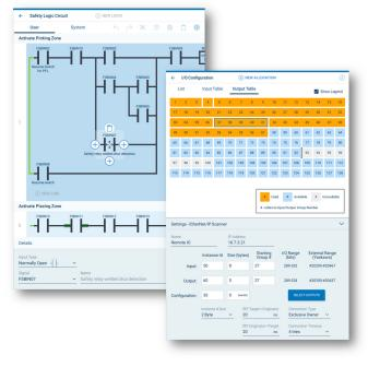
Graphical editors enable user to quickly configure system I/O and safety logic.
