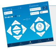
Smart Frame's patented technology determines the user's orientation relative to the robot. This eliminates the use of conventional coordinate (X, Y, Z) frames and utilizes intuitive natural language directions for easy command of the robot movement.
