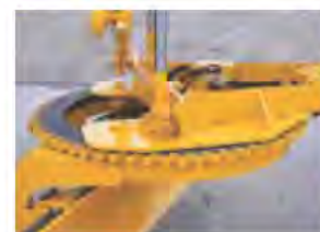
1,339 mm gear driven circle with "A" frame allows 360° blade rotation
