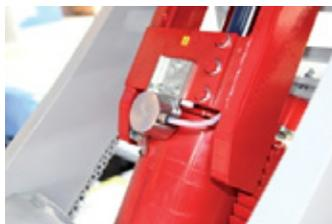
Mechanical safety locks secure the lift while it's working. Piston air is used for the opening of mechanical safety locks.
