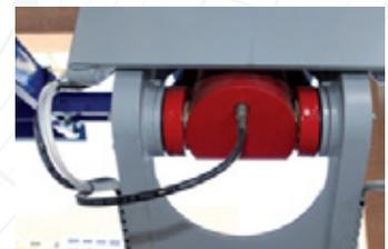
Burst valve inserted at the back of each lifting piston with hydraulic hose for high pressures, and 5 different pressure relief valves.
