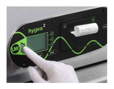
Every cleaning cycle can be recorded either in hard copy via the integral printer or electronically through a combination of the built in MC card port.
