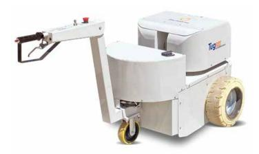
The Tug Rise pedestrian operated electric tug has been designed to tow on slopes or ramps, and is capable of towing up to 1 tonne on a 15 degree ramp with ease, or up to 5 tonne on a flat surface.
